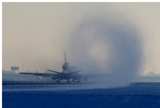
Figure 4: Wakes created by a landing heavy MD-11 (Source: Wikimedia )
